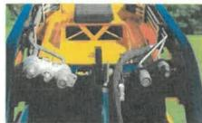
**HYDRAULIC BOOST.** The S925TX comes standard with a dual hydraulic auxiliary system with high flow to power the most demanding attachments and a low flow to give the operator maximum control.
